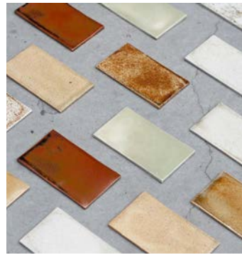
From top left to right: Agne Kucerenkaite's glaze research tiles, using pigments made from industrial metal waste; 'Karipot' from Tiipoi's 'Longpi Cookware' range, made from river clay and serpentine; Sinae Kim filtering residual solids of human urine to create ceramic glazes for her 'Urine Ware'
