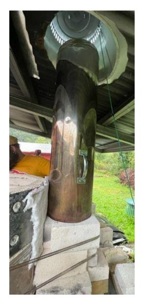
Here you can see the added 8" insulated stove pipe. We were able to fire to cone 10 in 3 hours with a 3' stove pipe. If you have a larger kiln body a 4' pipe or added brick layers may be necessary. This chimney could also be constructed from soft brick as the insulation increases the draw.
