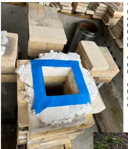
You can place tape upside down around the heat riser opening and set the kiln lid on it to determine where to cut. A cardboard template cut to ~7"x7" and set about 3" in from the edge of the bottom would also work. We cut the brick with a jigsaw and old blade after drilling holes in each corner.
