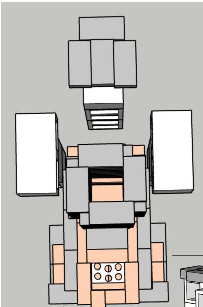
This step adds the concrete block supports for the kiln body and the chimney.
