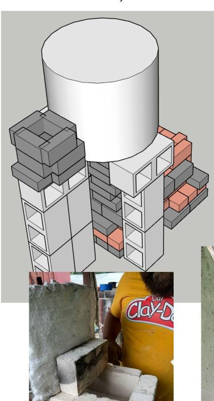
This layer of soft brick requires some notches to be cut and a brick shortened. Again, the hole should be about 7"x7". The chimney will sit on top of this layer. We added and 1' square of kaowool between this layer and the kiln to create a nice seal before adding the stove pipe.
