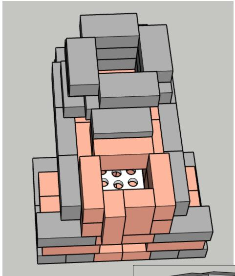
The third layer of the heat riser. This offset should be similar to the bricks to layers down (Layer 6).
