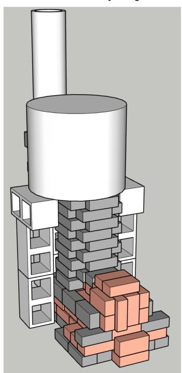
Hard bricks are placed over the firebox opening and the fuel (the skinnier the better) is fed in from the top. This creates a "self-feeding" fire that burns from the bottom up.
