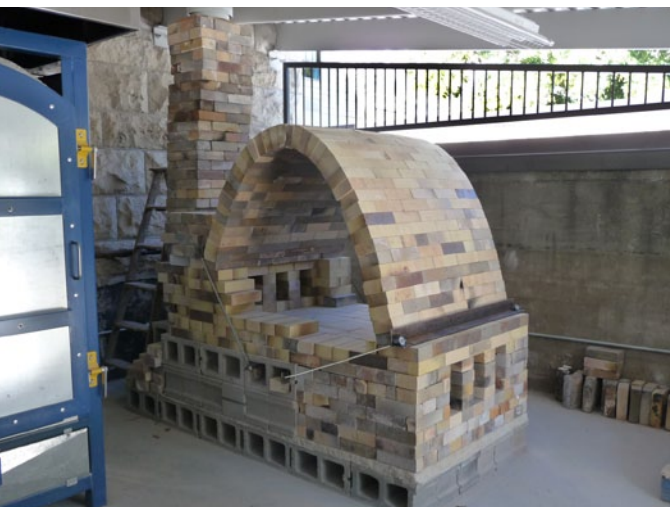
Top left: Figure 6. The soda kiln's intake and exit ports were built oversized and to standard size brick dimensions for easy modification of the burners.
